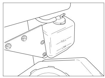
Figure 17. Radiator Expansion Tank
